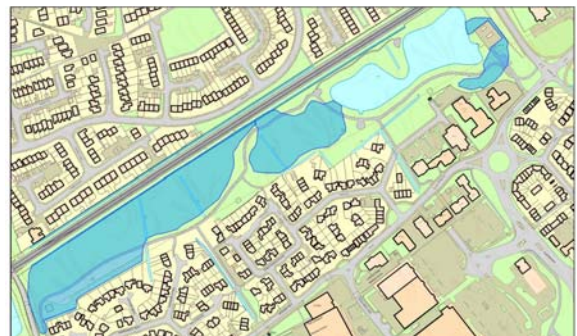
Figure 36: Flooding extent of green open space from the Summer Lane Ponds overtopping
